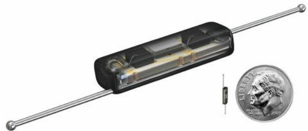
Figure 2. The SAVI SCOUT® reflector. Size comparison.
